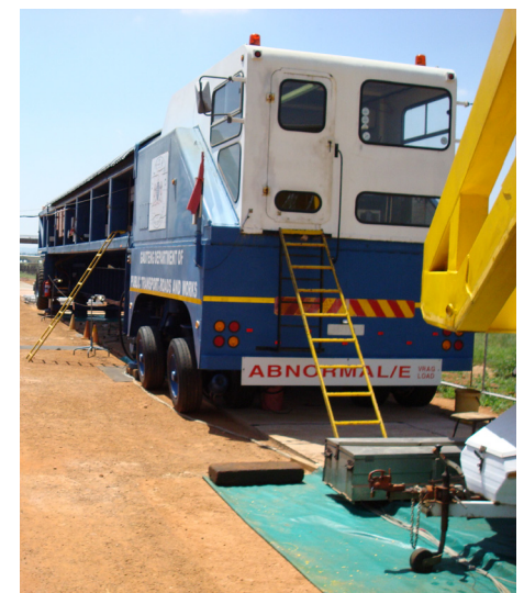
The heavy vehicle simulator used for testing the ultra-thin, continuously-reinforced concrete technology
