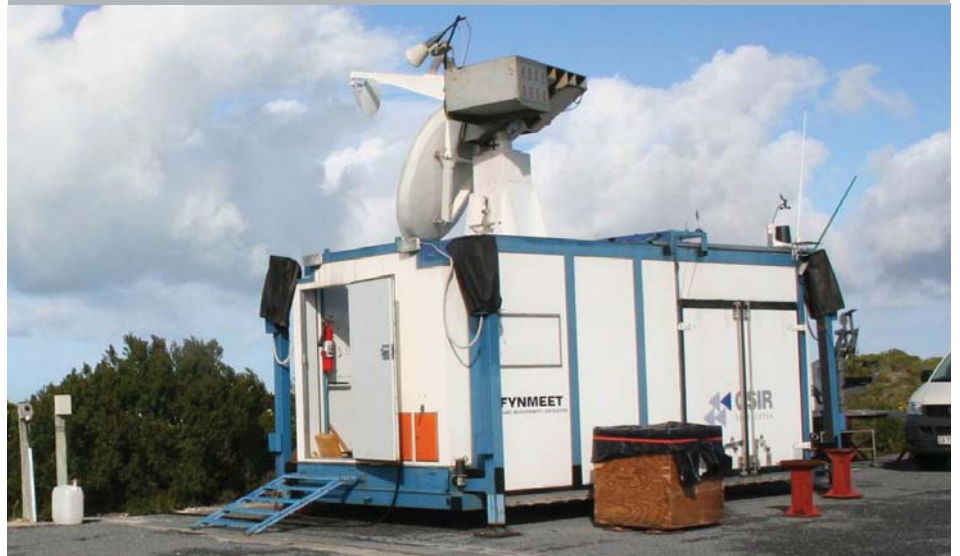
The Fynmeet radar measurement facility deployed at the Overberg Test Range to measure the radar characteristics of small boats in sea clutter during August 2006.
