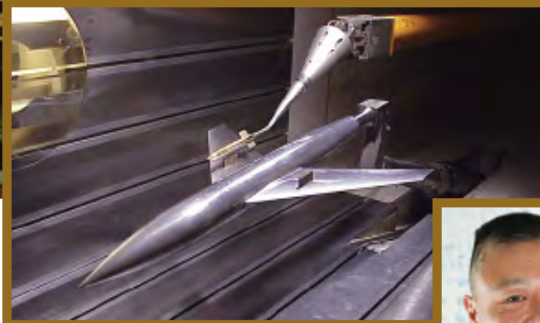
The release of a store off a South African Air Force Hawk is simulated in the image top left. Above: Two CSIR engineers prepare for the testing of a model aircraft in the CSIR medium-speed wind tunnel. Pictured in the inserted photograph is a store release validation, undertaken in the medium-speed wind tunnel at the CSIR, using generic parent and store models. Sean Tuling (right) of the CSIR says an aircraft's aerodynamics influences the trajectory of a weapon when it is released
