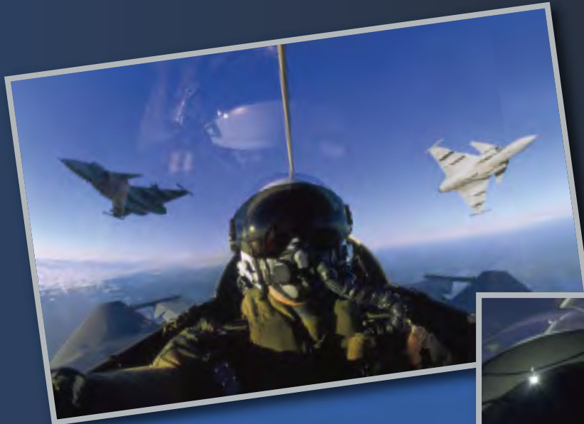
The Cobra helmet, as used in the SAAF's Gripens, can display critical data directly onto the visor and tracks where the pilot is looking. Displaying information on the pilot's visor means that the pilot does not have to continually glance down at the cockpit instrumentation while the head tracking allows aircraft sensors to be automatically directed towards targets of interest. Images copyright Gripen International Photographer: Katsuhiko Tokunago
