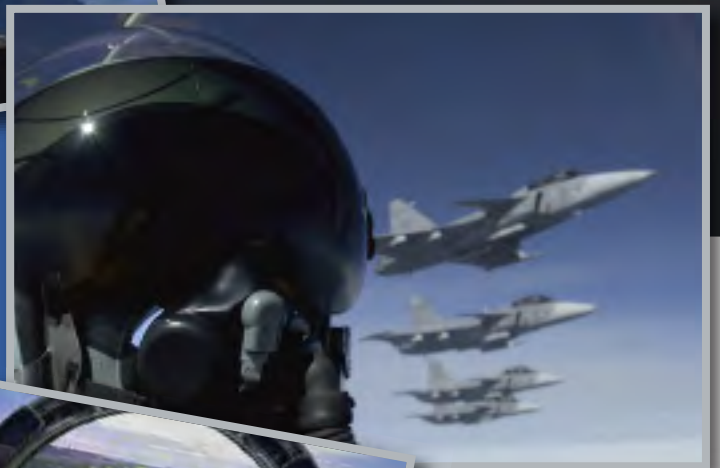
The Cobra helmet, as used in the SAAF's Gripens, can display critical data directly onto the visor and tracks where the pilot is looking. Displaying information on the pilot's visor means that the pilot does not have to continually glance down at the cockpit instrumentation while the head tracking allows aircraft sensors to be automatically directed towards targets of interest. Images copyright Gripen International Photographer: Katsuhiko Tokunago
