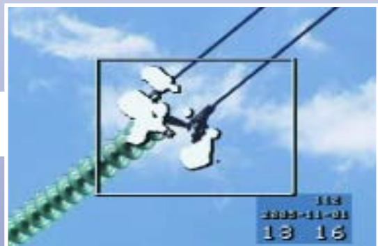
CoroCAM 504 in use with typical UV discharge overlaid on background image output
