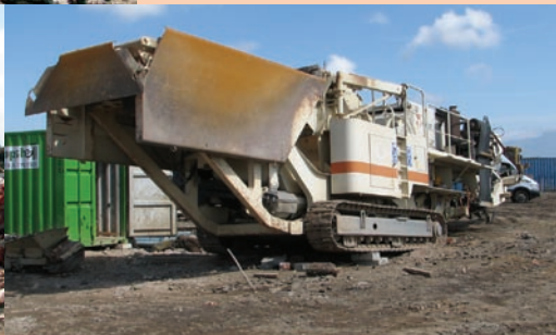
City of Cape Town re-uses tar remnants (left) as road surface at the Bellville landfill. Building rubble is crushed (see below) and used in road construction.
