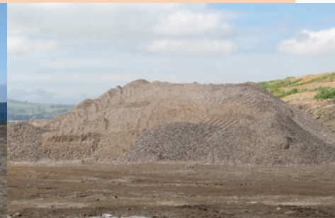
City of Cape Town re-uses tar remnants (left) as road surface at the Bellville landfill. Building rubble is crushed (see below) and used in road construction.
