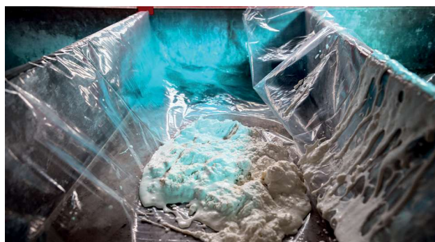
Metal-organic framework cakes are collected after mechanical dewatering using a pilot-scale filter press.
