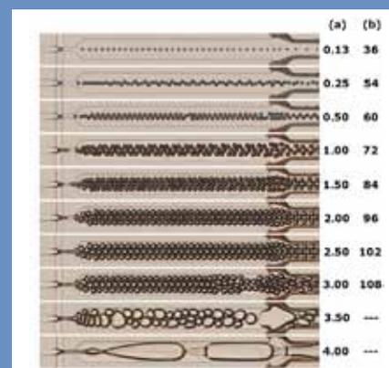
Droplets being generated in a flow focused microfluidic device. The frequency and size (b -  $\mu\text{m}$ ) of the droplets can be precisely controlled by varying the flow rate of the various fluids (a -  $\mu\text{l}/\text{min}$ ).
