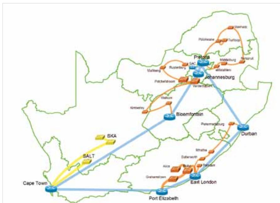
A map showing the SANReN national backbone in blue. Yellow lines indicate extensions under completion. The orange lines indicate future backbone extensions.
