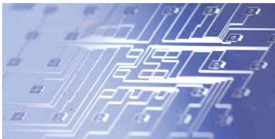
A typical microfluidic mould used for the manufacturing of devices.
