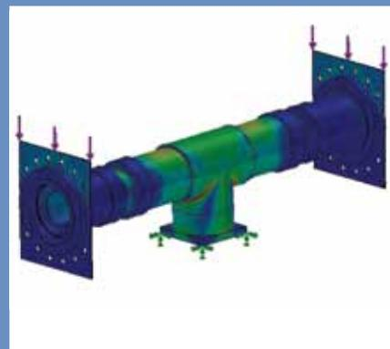
Predicted load distribution during development of the CSIR heliostat.
