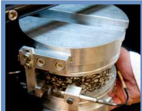
Shear testing of asphalt samples in the CSIR laboratory. Asphalt is a composite material, consisting of graded mineral aggregate (crushed rock) blended with a bituminous binder. It is commonly used in the construction of road surfaces, airport runways and parking lots.
