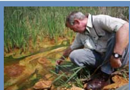
CSIR geohydrologist Phil Hobbs measuring the pH of acidic mine water decanting from abandoned mines in the Western Basin.
