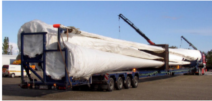
Figure 2: Example transportation of 3 x 45m wind turbine blades on extendible trailers
