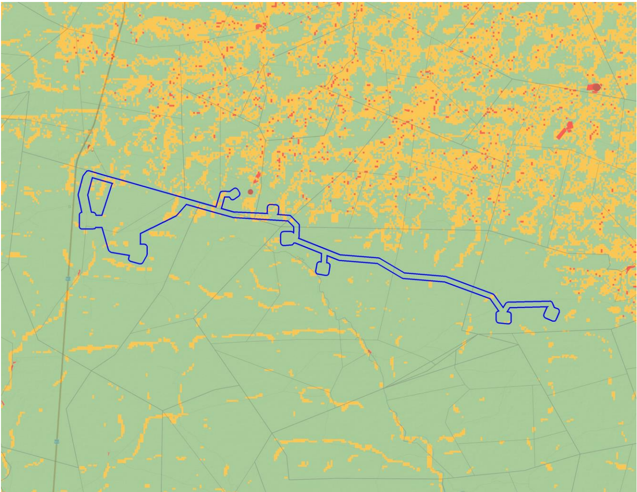
Figure 2. The proposed corridor in which the 7 power lines will be located (dark blue outline) overlaid on agricultural sensitivity, as given by the screening tool (green = low; yellow = medium; red = high).
