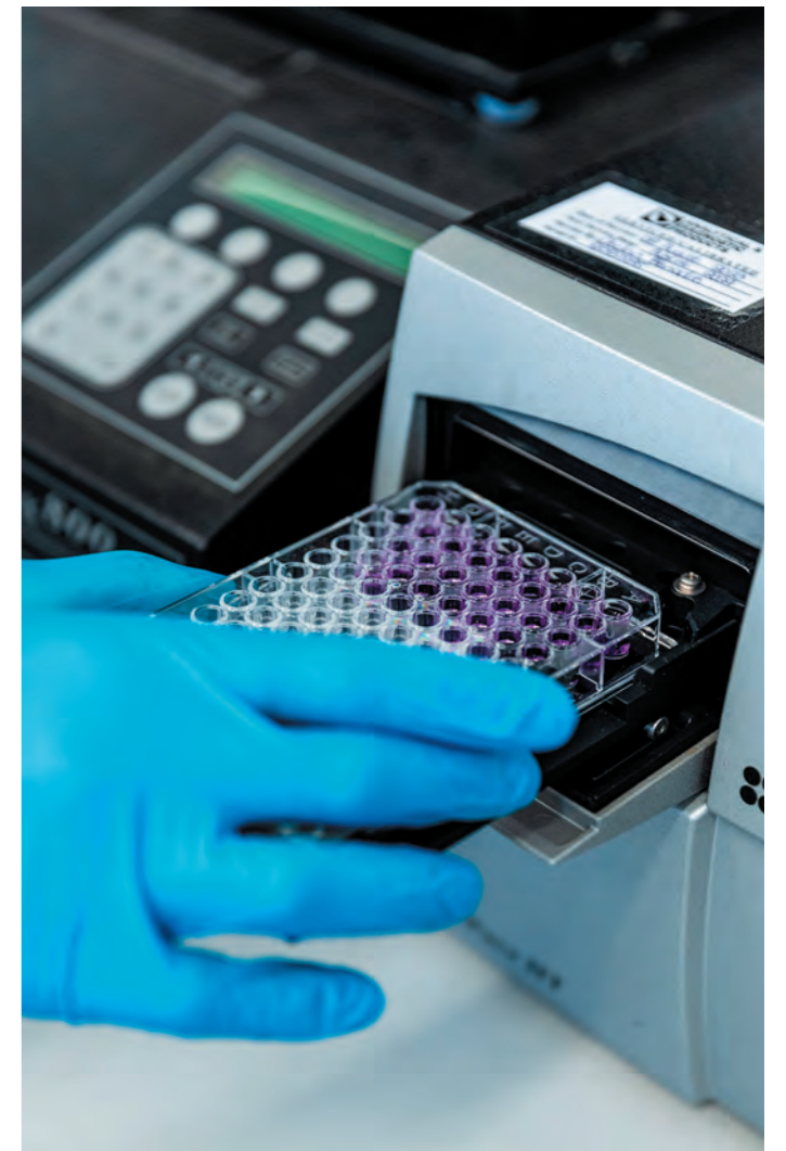
Protein extracts from patient urine samples being quantified using an ultraviolet-visible spectrophotometer.
