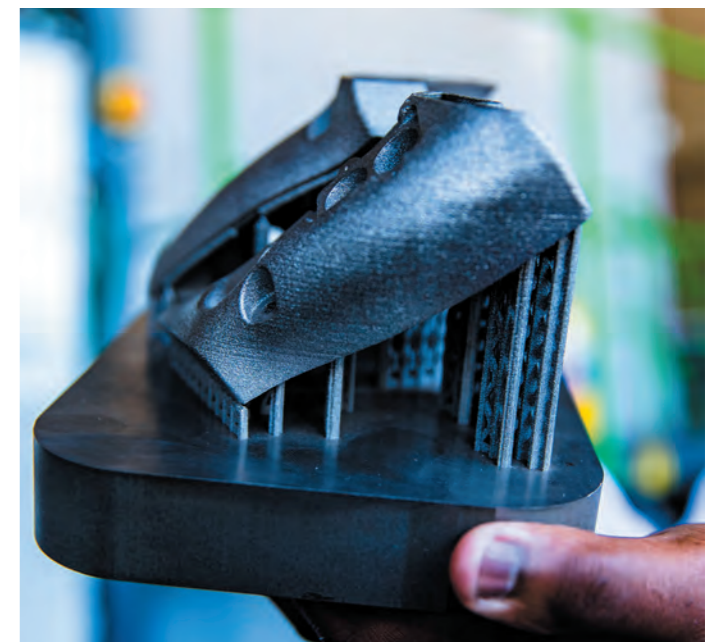
Nested build layout of a throttle grip, also from titanium alloy. A range of materials and techniques are researched and tested.
