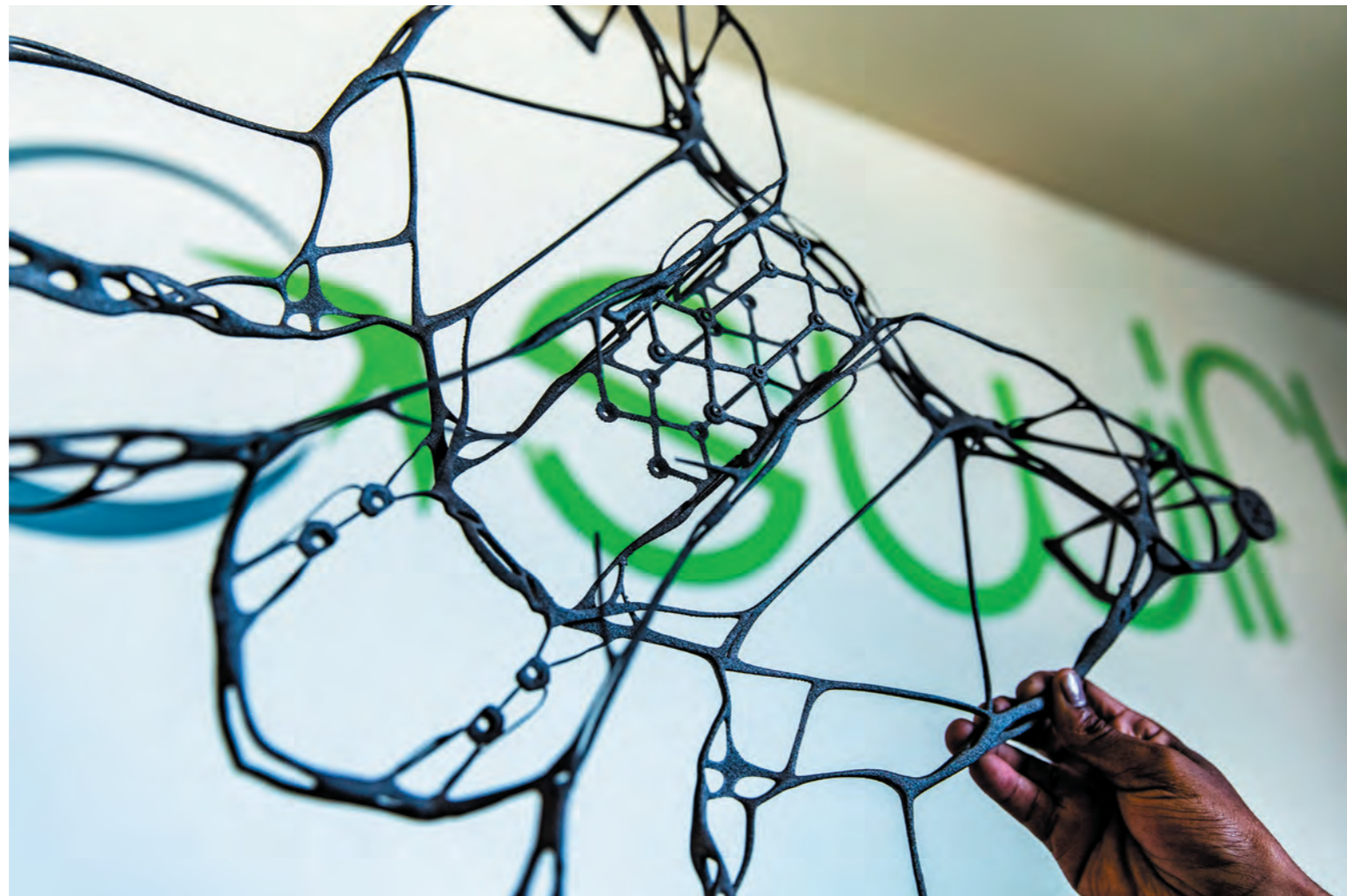
From the intricate to the heavy: An unmanned aerial vehicle frame benefits from the flexibility of 3D printing (above). A leading-edge turbine blade cover (50 cm in length) for an aircraft engine (below).
