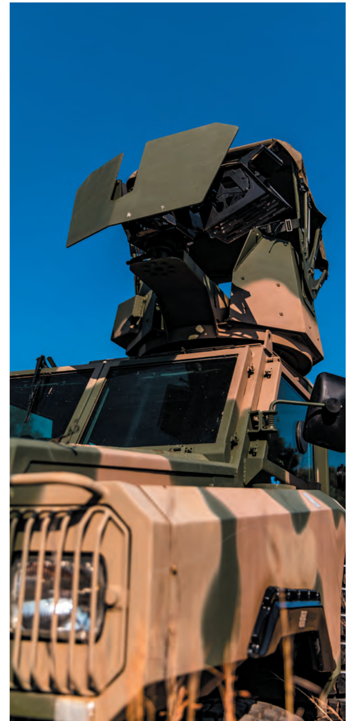
The CSIR-developed turret can be retrofitted to a range of different personnel carriers to provide protection to the gunner and a 360° arch of fire.
