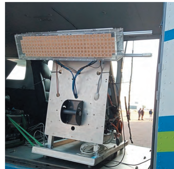
The CSIR C-Owl UAV synthetic aperture radar demonstrator installed on a Cessna 208 for flight tests.
