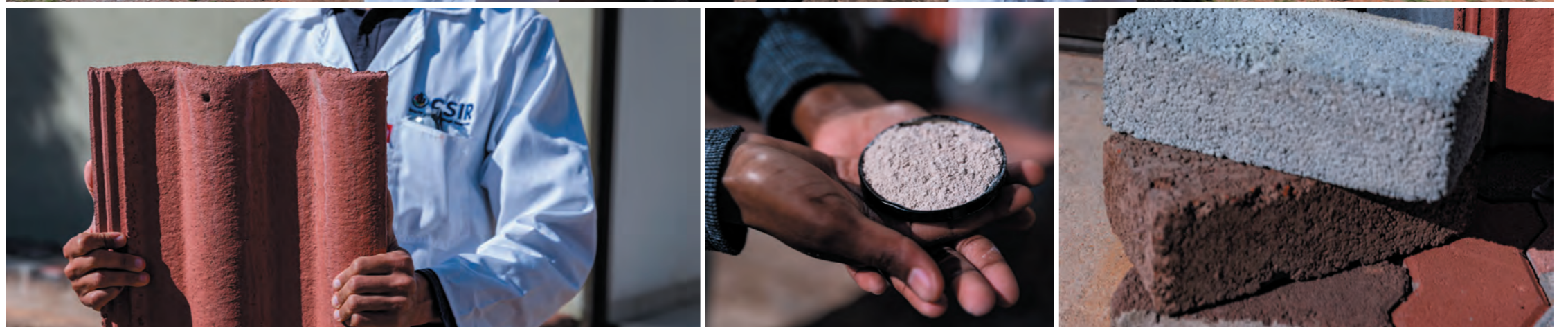
Top: CSIR researchers at an experimental site where the technology was tested. Left: A concrete roofing tile industrially manufactured from a CSIR-developed cement blend. Above: A sample of the CSIR 'green' cement blend. Right: Stock bricks made using CSIR 'green' cement blends and different aggregates.
