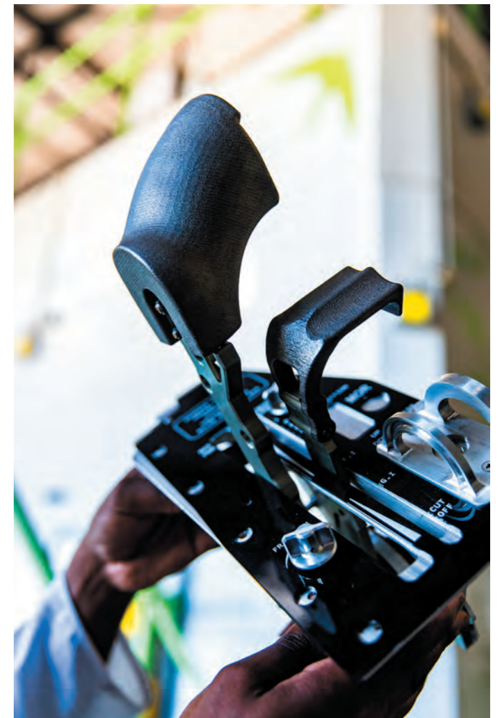
A light aircraft throttle grip printed in titanium alloy. 3D printing has found its way into several industries including power supply, defence, mining, automotive and aeronautics.
