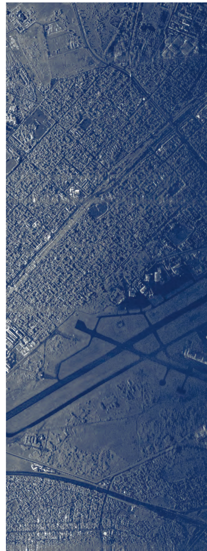
C-band synthetic aperture radar image created over Centurion, Gauteng in 2022, using CSIR C-band (5.5GHz) radar technology.
