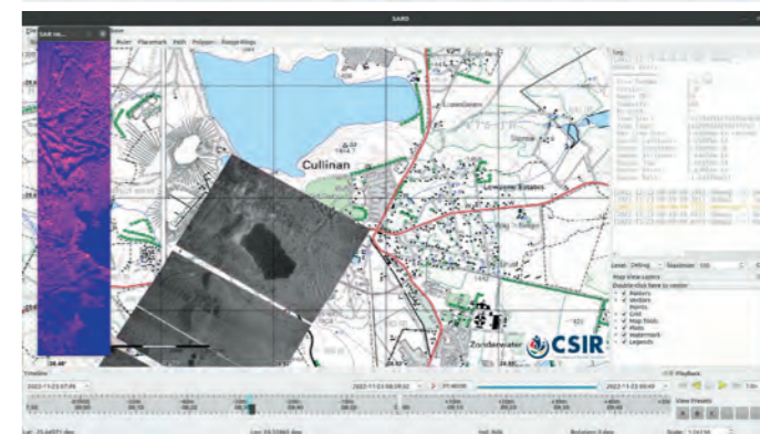
Above and middle: Doppler map and real-time synthetic aperture displays captured during flight tests.
