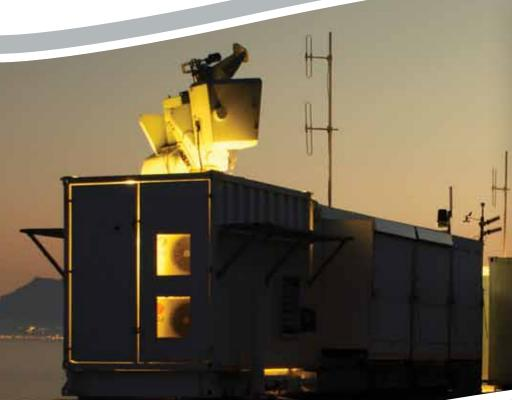
MECORT plays an important role as the research vehicle for advanced upgrades and algorithms on the Optronic Radar Tracker (ORT) on the Valour class Frigates. The system was already successfully utilised to support research into innovative multipath mitigation techniques and small boat detection techniques.
