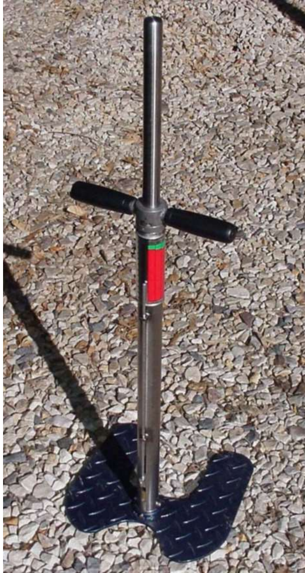
Figure 13: RCCD Device for indicating proper compaction
