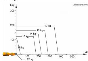
The KR 16 R1610-2 is designed for a rated payload of 16 kg in order to optimize the dynamic performance of the robot. With reduced load center distances, higher loads up to the maximum payload may be used. The specific load case must be verified using KUKA.Load. For further consultation, please contact KUKA Support.
