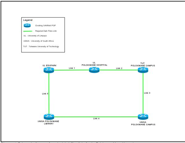
Diagram 1: Schematic diagram of required dark fibre links for the Polokwane Metro Network
