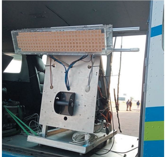
The CSIR C-Owl UAV synthetic aperture radar demonstrator installed on a Cessna 208 for flight tests.
