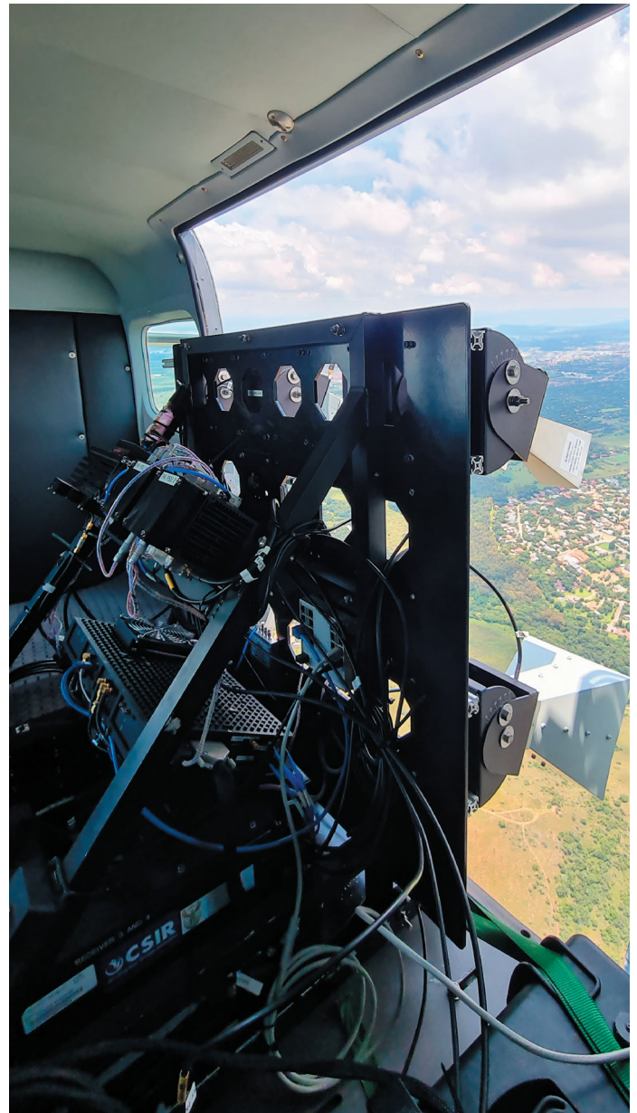
View from the aircraft while flight-testing the CSIR C-band synthetic aperture radar airborne test facility.
