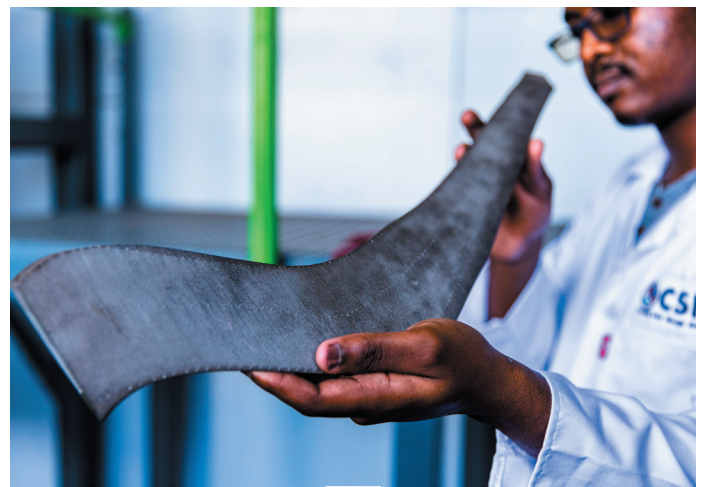
From the intricate to the heavy: An unmanned aerial vehicle frame benefits from the flexibility of 3D printing (above). A leading-edge turbine blade cover (50 cm in length) for an aircraft engine (below).
