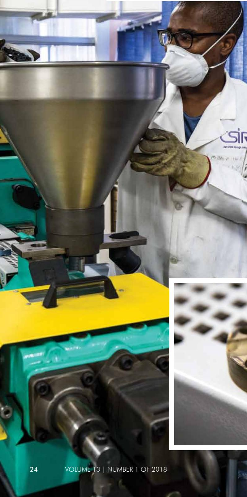
The CSIR has developed a customised metal injection moulding technology platform that allows for the cost-effective mass production of complex near-net shaped components from fine titanium powder. This technology platform makes it possible to overcome the geometrical and productivity limitations of traditional production techniques.
