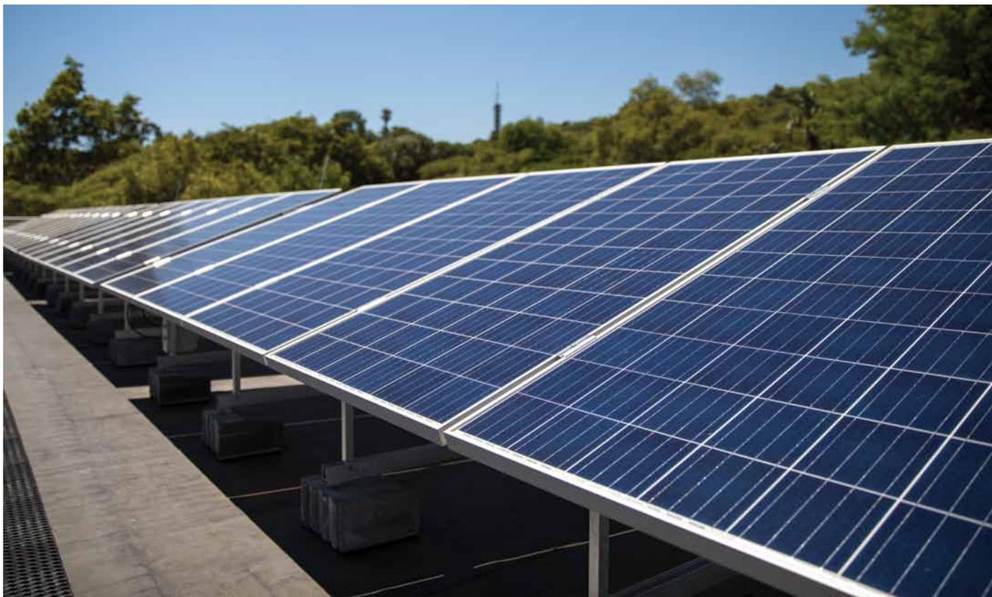
◀ Left and above: The CSIR outdoor testing system is used for research on solar system design and optimisation in realistic outdoor environmental conditions. (Inset) The performance of the system is correlated to meteorological readings derived from a weather monitoring system.
