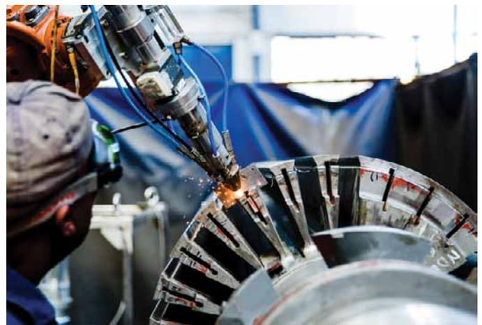
◀ Left: The CSIR’s 3D laser-cutting capability offers a cost-effective solution for manufacturing of formed components. ▲ Above: The CSIR has built a strong competence in laser-based refurbishment based on laser cladding technology. This technology is best suited for the repair of large and high-value components, such as generator rotors.
