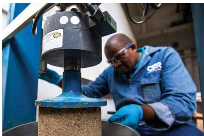
◀ Left: Samples to be tested using a dynamic shear rheometer, which is used to characterise the viscous and elastic behavior of asphalt binders at medium to high service temperatures. (Inset) CSIR lab technician Nomashaka Hawes uses a flash point tester to determine the temperature at which the sample will ignite.
