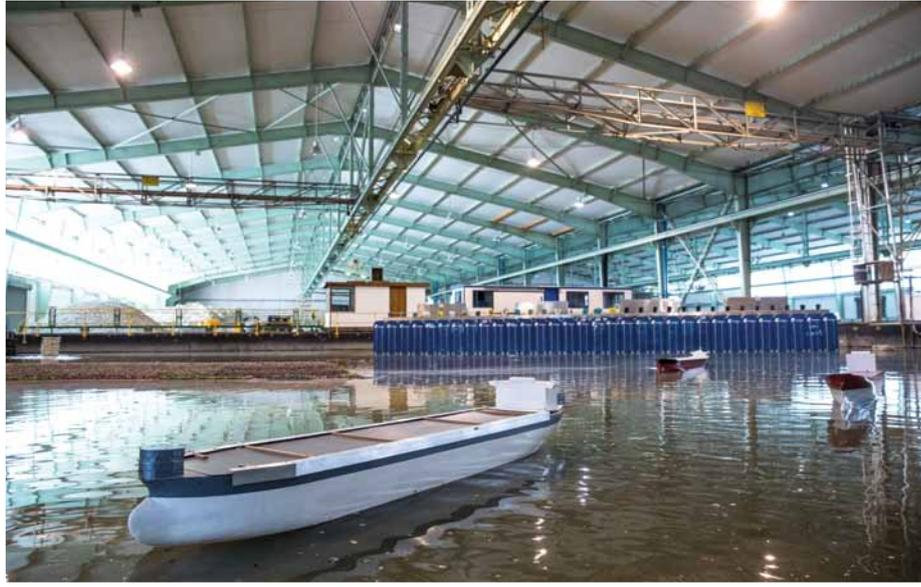
The CSIR's coastal and hydraulics laboratory is used as a design tool where engineers and scientist can build small-scale versions of planned coastal infrastructure and its surrounding area. The coastal processes and wave conditions are then simulated to test the performance of the planned infrastructure as well as the unintended impact such structures may have on the surrounding coastline and coastal processes. The impact of future climate change can also be tested in these physical models.
