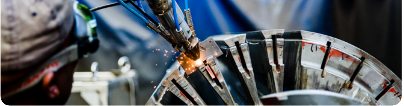
Restoration of the metallic surface of a generator rotor through laser cladding.
