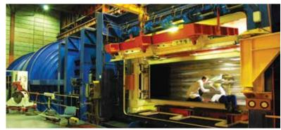
Wind tunnel which simulates flight conditions in a controlled environment to provide a test, measurement and evaluation service to the SA aeronautical industry
