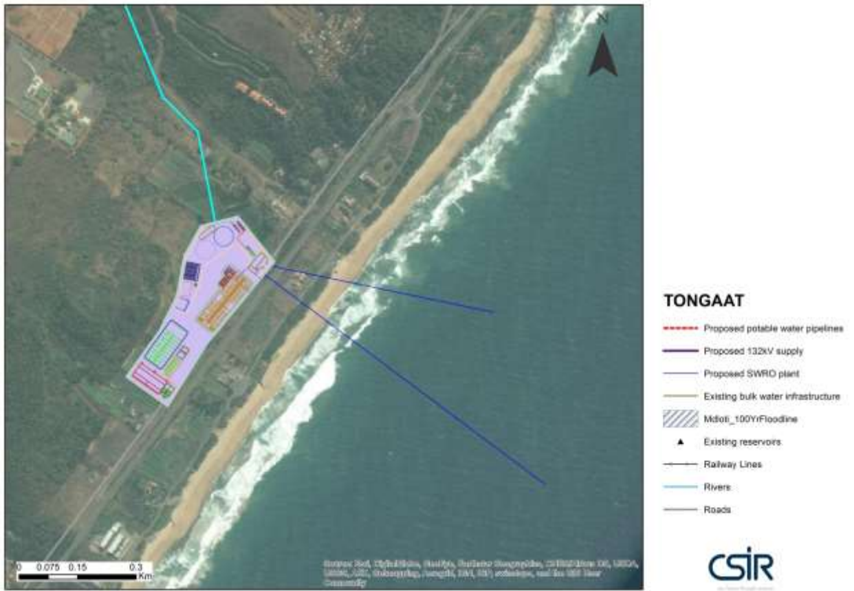
Figure 1: Overall Proposed Layout of the Desalination Plant and Associated Marine Infrastructure at Tongaat.
