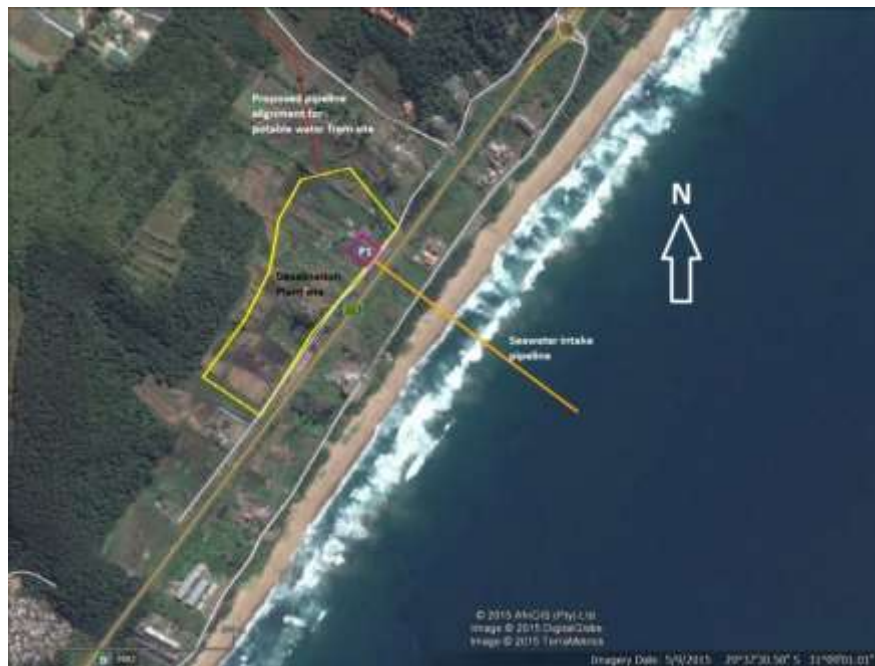
Figure 8-1: GOOGLE 2015 view of the proposed desalination facility at Tongaat, showing locations of proposed pump station (P1), desalination plant boundary (yellow polygon) and position of proposed seawater intake pipeline (tunnel) (orange).
