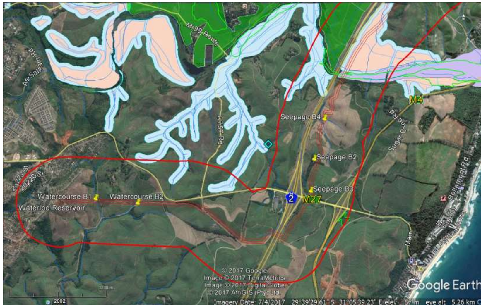
Figure 8-12 : GOOGLE images of the proposed La Mercy to Waterloo pipeline route (50m corridor shown as three red lines; 1000m corridor shown as thick red line) – Waterloo Reservoir to the Mdloti River crossing section, with 500m buffer around proposed pipeline route.
