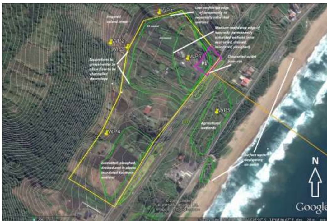
Figure 8-4A: 2015 GOOGLE Earth image of the proposed desalination site, with 2 metre interval contour data and estimated extent of wetlands (green polygons) within the two basins in the desalination plant area. Purple polygon indicates proposed pump station site; the yellow polygon indicates the proposed desalination plant site boundary. “WP” prefix indicates augered points referred to in text.
