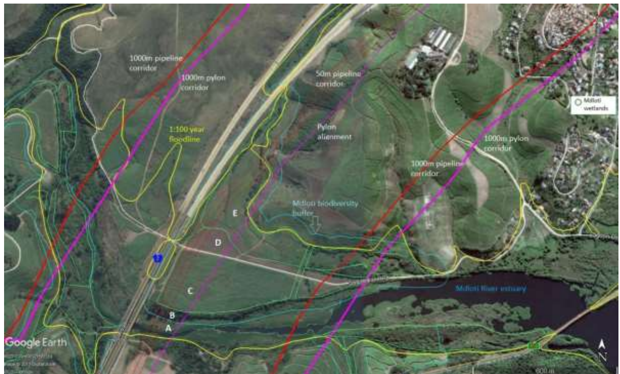
Figure 8.10: Near-view of proposed pipeline (Alternative 1) and powerline (Alternative 2) crossing of the Mdloti River estuary
