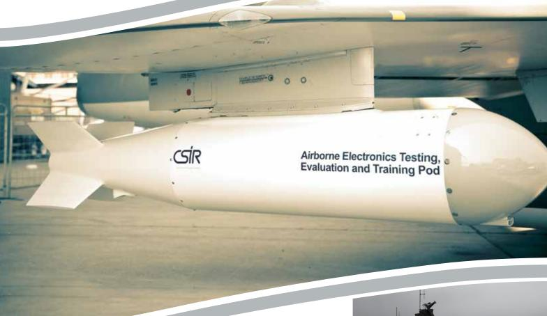
Inundu is a multi-purpose electronics pod for airborne Electronic Warfare (EW) and Radar test evaluation(T&E) and training applications. The modular payload can be re-configured for various research, development, test, evaluation and training scenarios.
