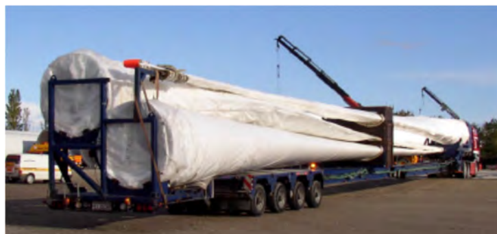
Figure 9: Example: 3 x 45m Blades on extendible trailers
