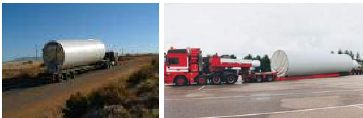
Figure 2.8: Tower section being transported.
