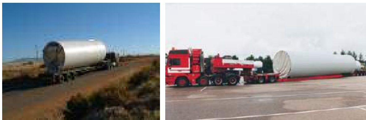
Figure 2.9: Tower section being transported.
