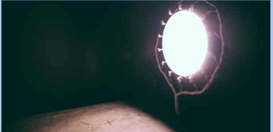
An integrating sphere source generates a uniform radiance for a hyperspectral camera and is used for satellite calibration and camera non-uniformity characterisation.
