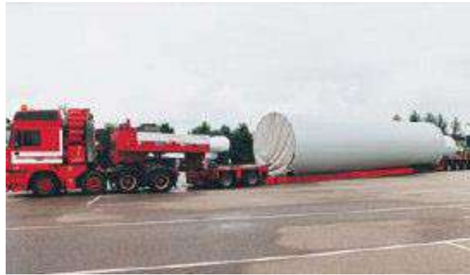
Figure 2.8: Tower section being transported.
