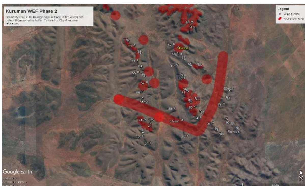
Figure 5.13: The location of high sensitivity areas in the WEF development area. The turbine indicated in yellow falls within the no-turbine zone. Other infrastructure is allowed within the high sensitivity areas.
