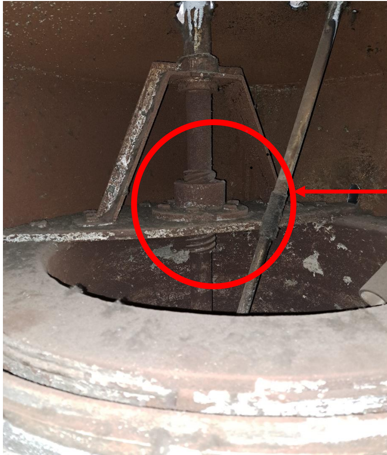
Fig 2: Screw type spout operating mechanism
