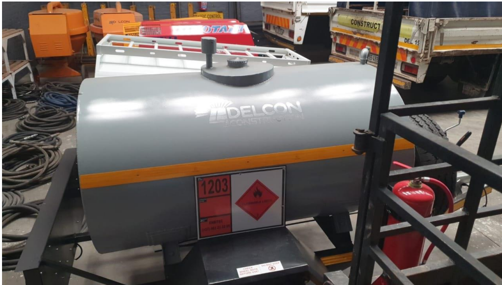
Figure 11: Example of a mobile fuel trailer for fuel transport and storage.
