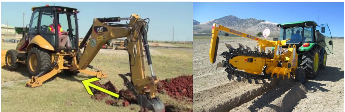
Figure 2: Example of machinery used to dig trenches -Tractor Loader Backhoe (TLB) (left) and Chain Trencher (right).
