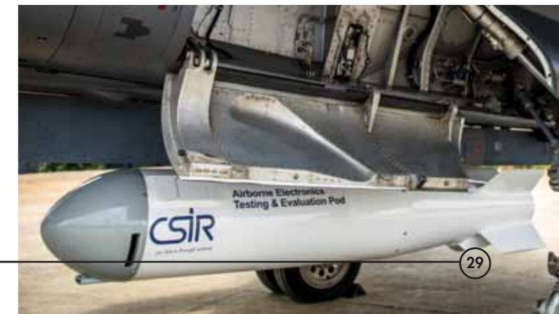
▼ Below: (left) The ram air turbine underwent tests in the CSIR's medium speed windtunnel to validate the levels of power it was able to generate over the full flight envelope of the pod. (Right): The pod was also tested on a Mirage F1 fighter plane.
