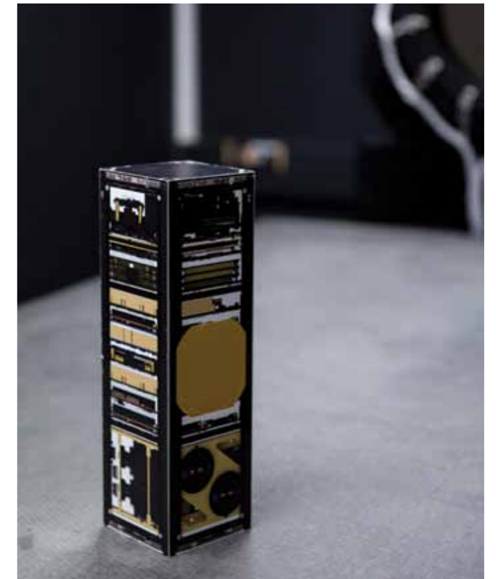
▲ Above: (left) A 3D printed plastic model of the K-line camera. (Right) A mock-up of the 30 x 10 x 10 cm ZA-CUBE-2 satellite with the K-line camera at the bottom of the cube stack.
