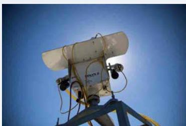
> **An outdoor solar photovoltaic module test bed installed on the roof of one of the buildings on the CSIR campus in Pretoria. (Inset) A dual-axis tracker used for measuring direct normal irradiation and direct horizontal irradiation. These solar resource measurements validate short-term energy forecasts.**
