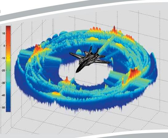
SigmaHat is based on asymptotic (high frequency) EM calculation techniques and can be used to calculate the RCS of electrically large complex 3D objects such as aircraft, land vehicles and ships.
