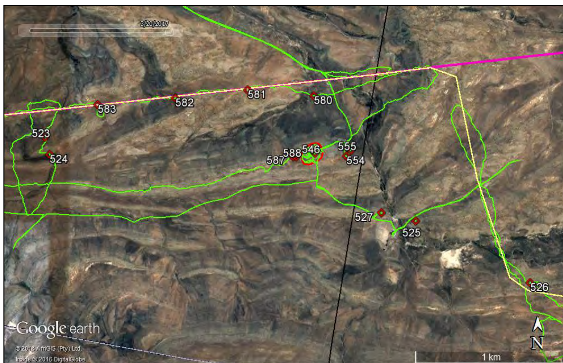
Figure A2.2: Aerial view of the eastern part of Alternative 1. The yellow/pink line indicates the power line routing and the red numbered symbols are waypoints. The green lines are survey tracks.
