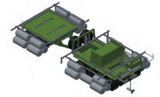
Geckos were fitted with flotation devices and additional propulsion so that they could go from the road into the water. These adapted vehicles were used to rescue flood victims who are stranded in trees and on top of buildings.
