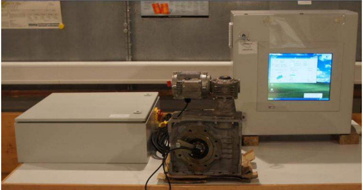
Figure 2: Tracker and DC combiner test set-up
